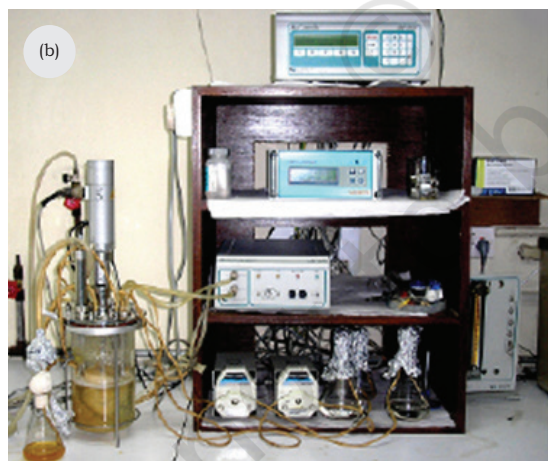
Fig. 10.1: (a) Diagrammatic representation of the design and components of a typical bioreactor (b) Photograph of a laboratory bio-reactor
